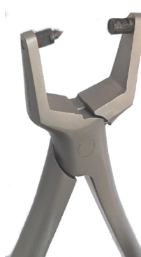
10/3400 Peening: pointed & cupped tip used for flaring screws (temple & hinges) to prevent them from loosening, with sping handles
